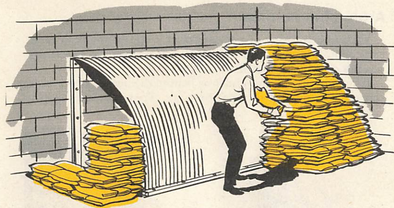
This four-person basement-corner shelter is made of curved asbestos-cement sheets which are covered with sandbags. Materials cost about $125.
